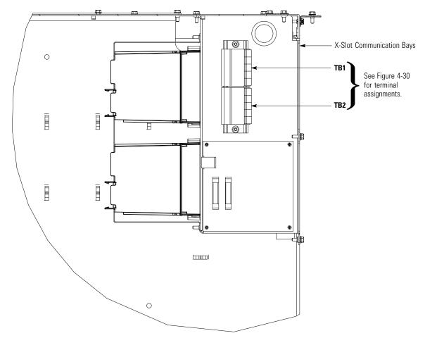
Figure 4-28. Interface Terminal Detail
